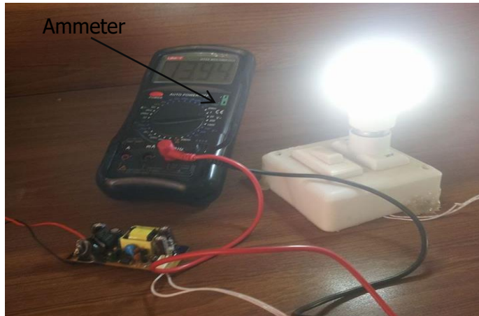
FIG 16 OUTPUT VOLTAGE OF LEDS LAMP
