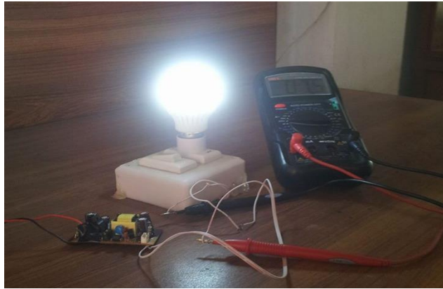
FIG 20 CURRENT OF 7A ON AMMETER
